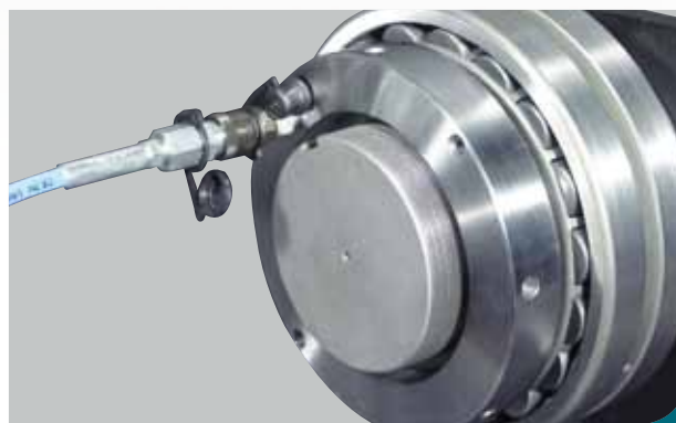
Extraction of the withdrawal sleeve with a hydraulic nut (reverse of the previous mounting)
